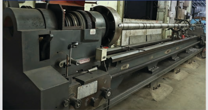
A German section bending machine that provides flexibility in forming the spiral (jalebi) limpet for fitting on bottom dish. This machine forms all sections - flats, bars, angles, channels, beams, square and rectangular pipes too.
