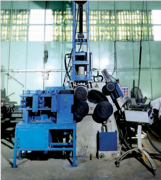
A European limpet coil forming machine for making JOINT FREE LIMPET COILS of maximum length , manageable for handling & fitting them on vessel. No Butt weld joints. Resulting safest and leakproof, even in case of double limpet coils, used for heating and cooling / chilling separately.
