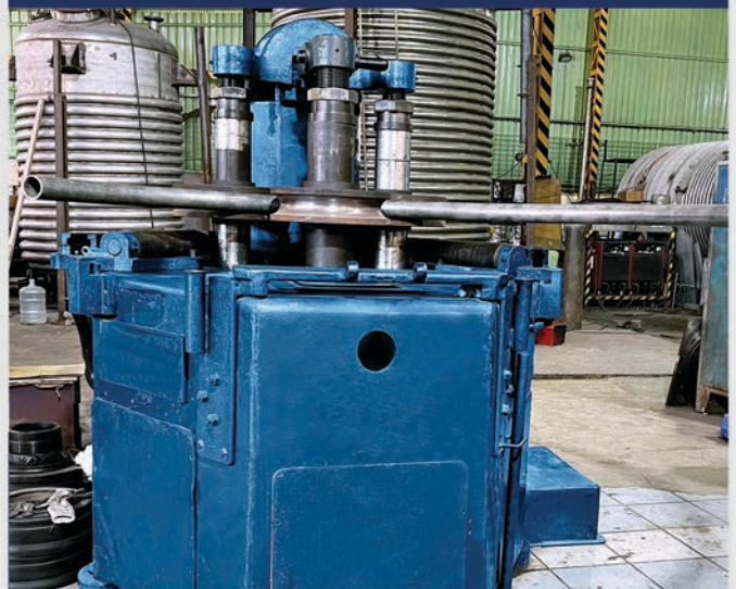
A German section bending machine that provides flexibility in forming the spiral (jalebi) limpet for fitting on bottom dish. This machine forms all sections - flats, bars, angles, channels, beams, square and rectangular pipes too.
