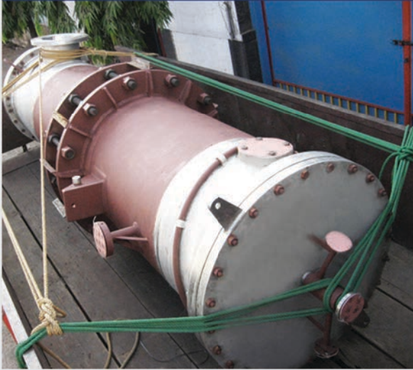
High Pressure Heat Exchanger
